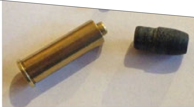
Can Wesson .177 Air Pistol Pellet Shell Design V7 Replaced the original (B) shell to enable the use of pellets for more accurate target shooting. Saves destroying the shells that come with the airgun. Rear of shell pushes the pellet into position. One dimension (in red) may need to be adjusted to firmly hold the pellet in place. Prototype is plastic, production will be brass or maybe copper.
